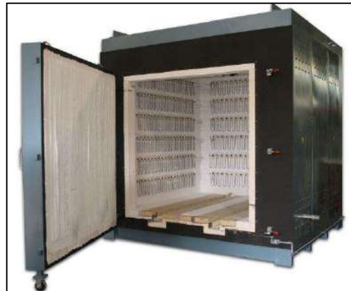
Figure 5 Electric batch kiln for ceramics (Blaauw)
