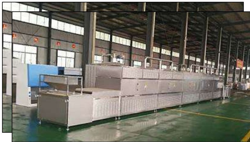
Figure 3 Microwave drying system for ceramic tiles [21]
